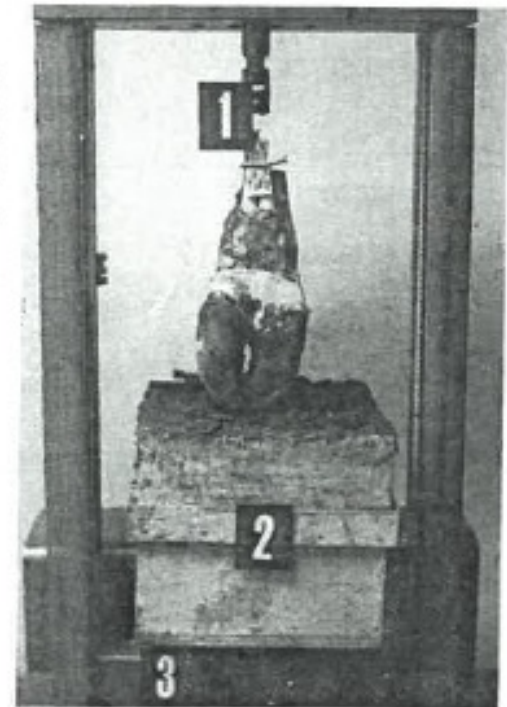
FIG. 1 Experimental setup—1) attachment of hoof to Instron unit. 2) mud box 3) attachment of mud box to Instron unit by means of the movable crosshead.
